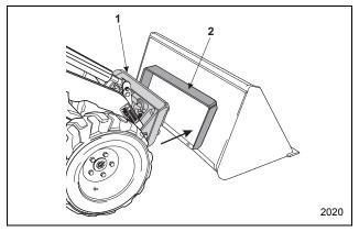
Figure 3–21 Non-powered Attachment Installation
